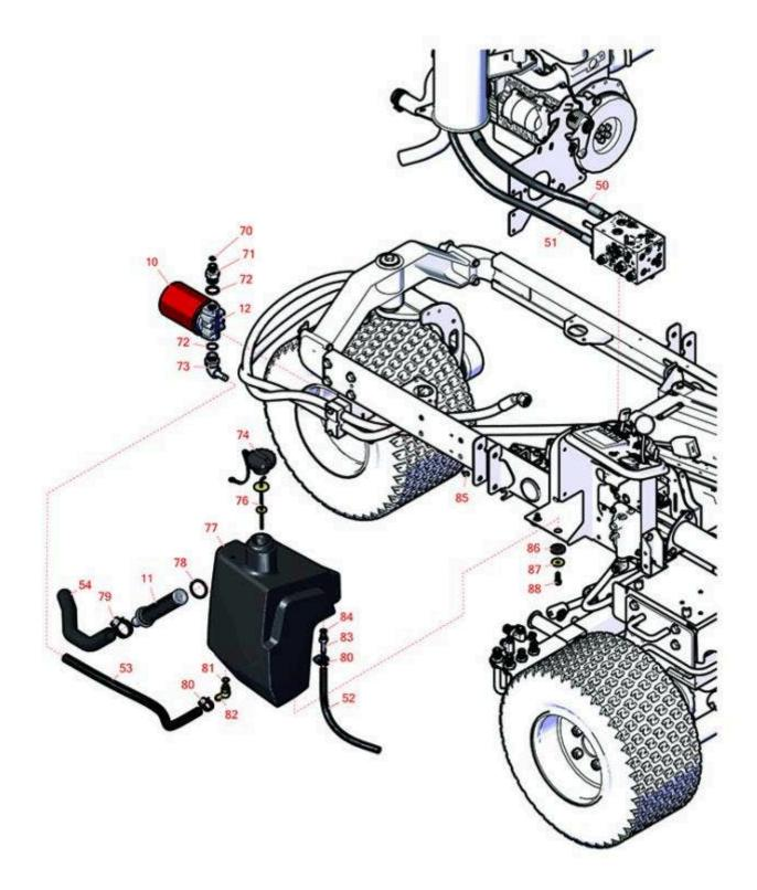
Traction Unit - Model 03174 Hydraulic Tank
